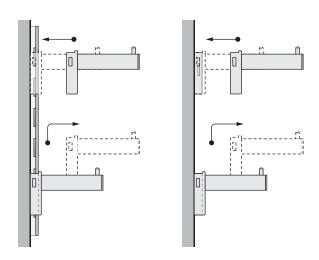
Single-sided and double-sided Beam profiles can be fastened on wooden panels (19-22 mm/0.748"-0.866"), glass panels (10 mm/0.394") or plexiglass panels.
